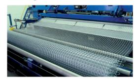
HUCKs anti-vandalism nets made from Dralo® have a distinctive contemporary and atractive appearance. These machine-made wire rope nets are formed into square meshing. Despite their robustness they retain their good looks and are soundproof.
