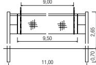
Volleyball posts made of special aluminium profile. Prepared for setting into ground sockets. Equipped with tensioning device with lever tensioner and chain, for easy application in play and leisure areas.
