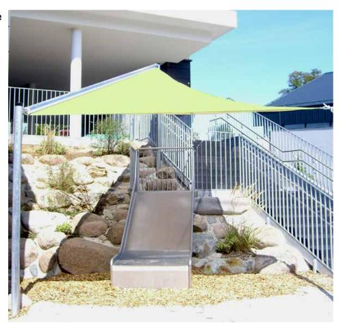
The posts are made from galvanised steel with plastic caps. The awning can be adjusted manually with a cable pull. The sun awning is made from mesh fabric "Soltis 86" (100% PES) with PVC coating. It is tearproof, durable and UV-resistant with a 86% UV filter protection. A winding roll with electric motor is available upon request.
