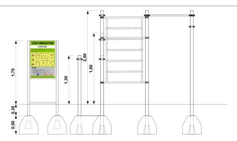
Each vertical column poured with semi-dry concrete C20/25 for 80 cm below ground level. Volume of one footing min. 0,125m³. Fundations are placed 30 cm below ground level, what prevent accidential or purposeful discovery.
