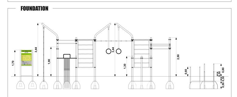
Each vertical column poured with semi-dry concrete C20/25 for 80 cm below ground level. Volume of one footing min. 0,125m<sup>3</sup>. Fundations are placed 30 cm below ground level, what prevent accidential or purposeful discovery.
