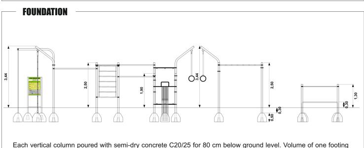
min. 0,125m<sup>3</sup>. Fundations are placed 30 cm below ground level, what prevent accidential or purposeful discovery.
