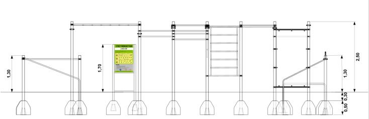
Each vertical column poured with semi-dry concrete C20/25 for 80 cm below ground level. Volume of one footing min. 0,125m<sup>3</sup>. Fundations are placed 30 cm below ground level, what prevent accidential or purposeful discovery.
