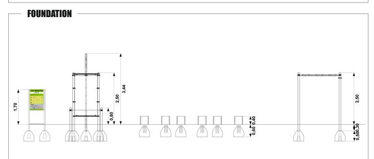
Each vertical column poured with semi-dry concrete C20/25 for 80 cm below ground level. Volume of one footing min. 0,125m³. Fundations are placed 30 cm below ground level, what prevent accidential or purposeful discovery.
